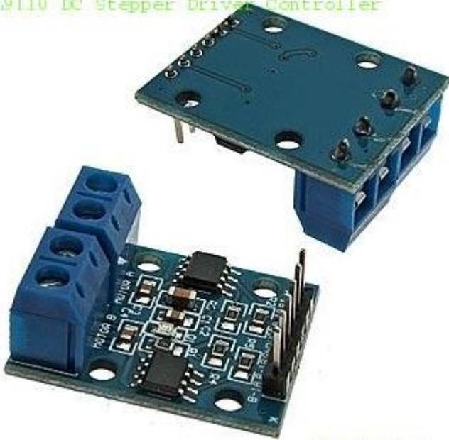
1. 2 onboard L9110S motor control chips
